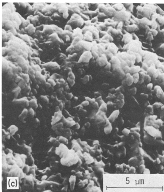
Figure 4 SEM micrographs of the microstructure of the silicon nitride. (a) Starting powder, (b) fracture of cold isostatically pressed specimen ( P = 200 MPa), (c) fracture of hot isostatically pressed \text{Si}_3\text{N}_4 with 10 wt% \text{Y}_2\text{O}_3 .
