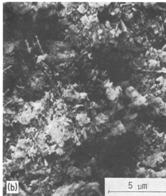
Figure 4 SEM micrographs of the microstructure of the silicon nitride. (a) Starting powder, (b) fracture of cold isostatically pressed specimen ( P = 200 MPa), (c) fracture of hot isostatically pressed \text{Si}_3\text{N}_4 with 10 wt% \text{Y}_2\text{O}_3 .
